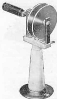
Neutralising Condenser, Cat. No. 1088. For HF circuits using low-capacity triodes. Maximum voltage 2,000 volts D.C. Capacity variation 1-8 mmfd. Frequentite pillar insulator mounting, insulated adjusting knob. Price 6/6
